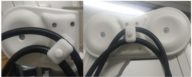
Figure 15: Cables secured in camera arm
