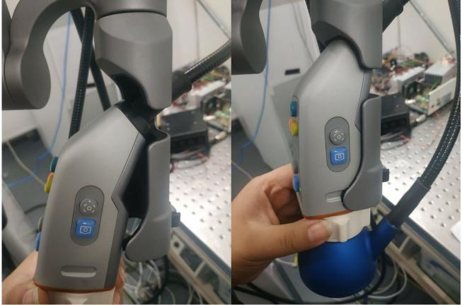
Figure 14: Camera positioned in arm gripper
