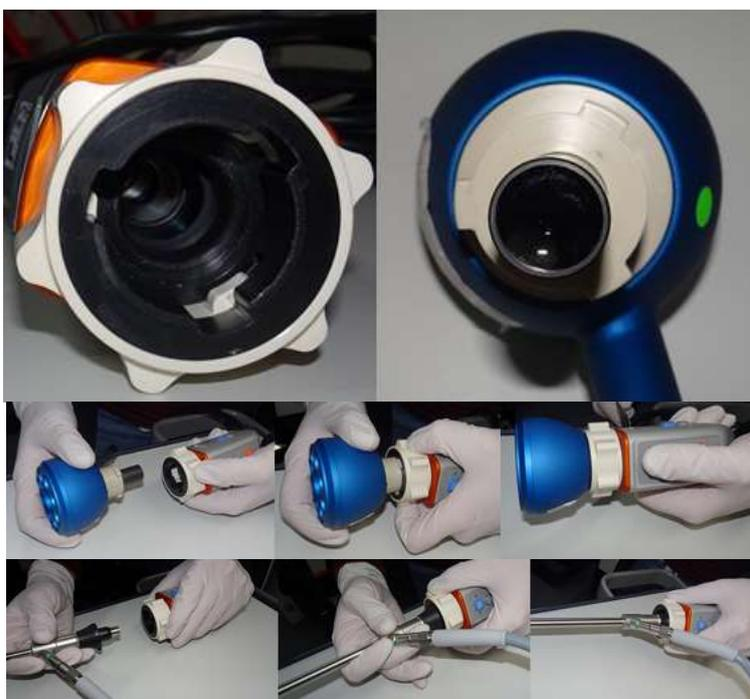
Figura 4: Connecting the ring light/Laparoscope to the camera
