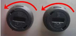
Figure 18: Replacement of the fuses
